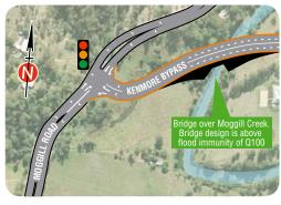
**Option B:** The bypass would link directly with Moggill Road to the south, with a signalised T-intersection to access Moggill Road to the north.
